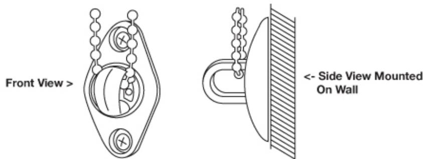
When installing the cord guide, make sure that the cord hangs loosely to optimize performance of the clutch and make sure that the cord connector passes through the guide with ease. Never twist or cross the control cord/bean chain, as this could damage the shade.
